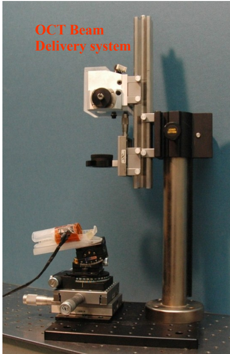
Figure.16. The beam delivery system of OCT and the heated cylindrical holder mounted on 6-axis positioner. (Uhlhorn SR, Borja D, Manns F, Parel JM. Vision Research 2008; 48:2732-2738)
